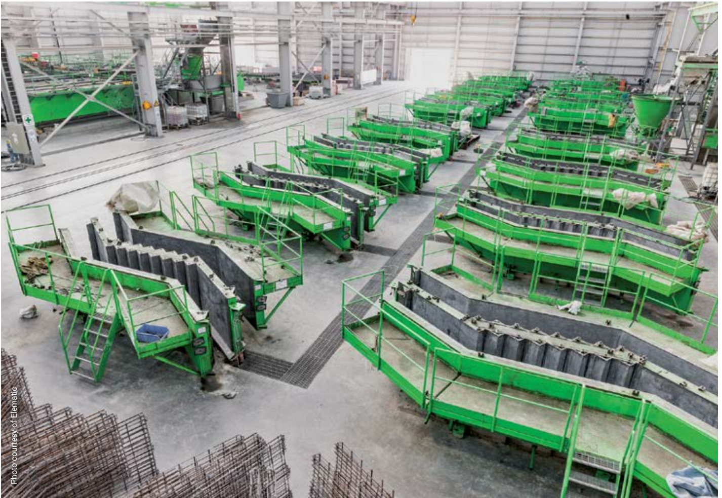
The battery mold plant houses 18 precast concrete stair molds.
