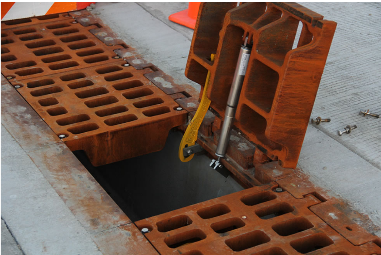
Hinged Trench by EJ with optional mechanical strut. Our stainless steel Lift Assist reduces the lift force required to open the grate to 35lbs or less.
