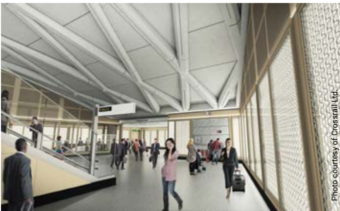
Architectural renderings depict Farringdon Station's public areas, which are clad with disc-shaped GFRC panels.
